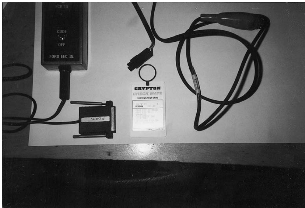
Fig. 3.16 The diagnostic lead and smart card for a Ford vehicle
